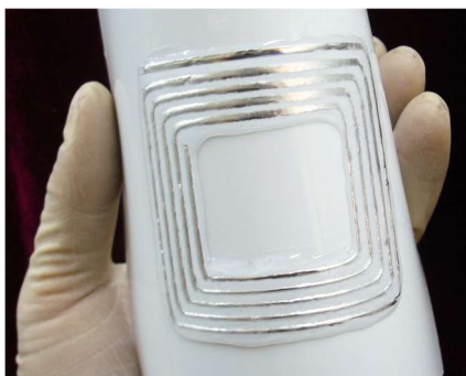
A radio-frequency-identification (RFID) antenna printed on paper.
